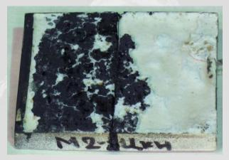
M2 material after combined thermal/skin friction action of plasma flow
