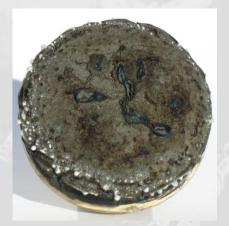
M2 material after a test in RF plasmatron facility in CO<sub>2</sub> plasma flow
