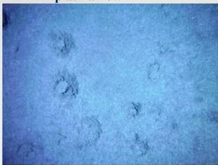
Microscopic view to the M2 ablated surface after erosion tests Torino 17 - 18 - 19 May 2016
