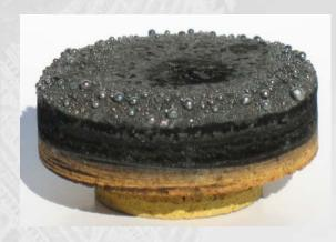
M7 material after a test in air plasma flow
