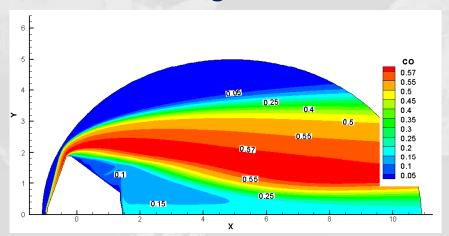
CO mass fraction field around the DM, H=60 km. Entry angle of 10.5°, cold Martian atmosphere
