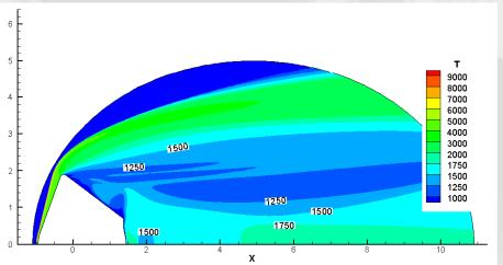
Temperature field around the DM, H=60 km. Entry angle of  $10.5^{\circ}$ , cold Martian atmosphere
