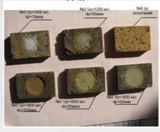
M7 material samples before and after erosion tests
